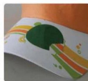
screenprint on visor 帽舌丝网印刷
